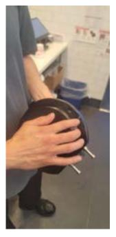
9)Place face plate onto shake machine lining up screws with holes
