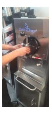
10)attach both screws one turn, once both are on then you can tighten them. Once they are tightened take paper towel and tighten more
