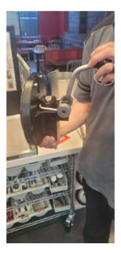
8)Spread lube around entire inner o-ring of face plate
