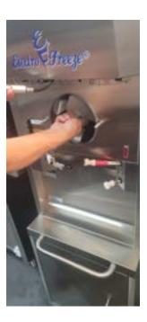
6)Fill white cap with lube and lubricate outside if it. Place in black face plate paying attention to the notch and that it lines up.
