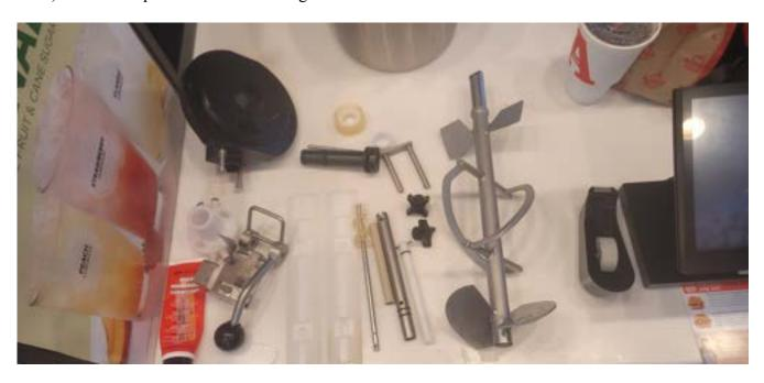
2) Lubricate the small ring (Whenever using the lubricant use it liberally, its cheap and will help machine last longer and your job easier.)
