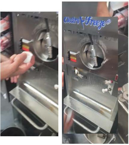
14)Remove the insides, make sure white cap is removed for proper sanitization
