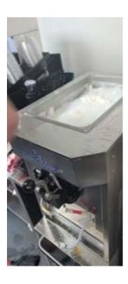
9) Break up large chunks of foam from shake mix and wipe sides to loosen film, if needed use paper towel to wipe sides
